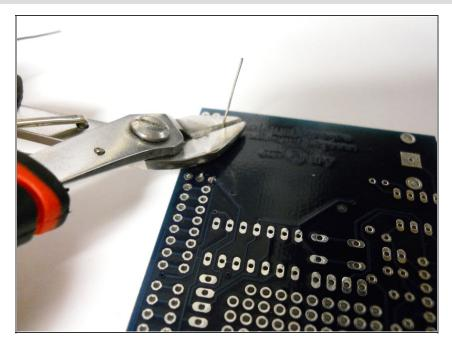
Make your soldering life easier by trimming the leads of the components after you solder them in.
